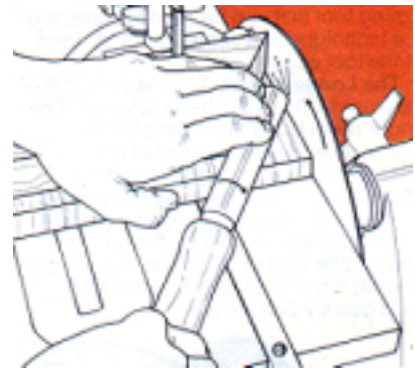
Fig. 5 Grinding Gouge. For this first step in a two-step procedure, firmly and slowly push the tool into the Disc with clockwise rotation following angle of jig and traveling through half of the Gouge bevel contour.
