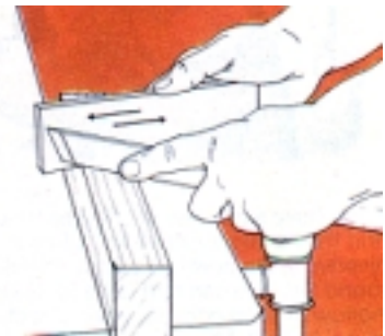
Fig. 6 Honing Lathe Chisels. Lubricate the benchstone and rub it on the Chisel bevel as you hold the tool steady.
