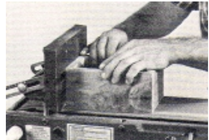
Fig. 4. After the glue has dried, sand the boxes. When using the belt sander, keep the box moving from side-to-side.
