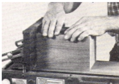
Fig. 6. Sand the sides flush after the glue has thoroughly dried.
