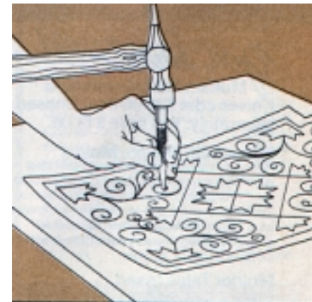
Fig. 5. Punching tin with a square-ground center punch.
