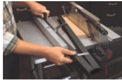
Fig 4: An Adjustable Taper Guide in use.
