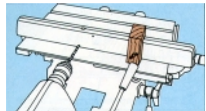
Fig 6: The Stop Block eliminates the need for you to mark each hole individually before you drill.
