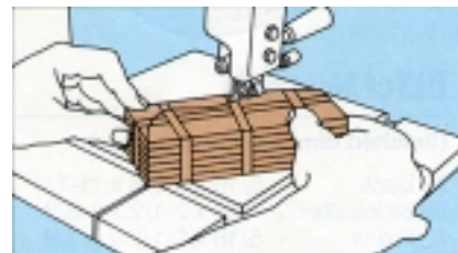
Fig 2: To "Pad Saw" your components, stack several pieces of thin stock on top of one another, tape them together and cut them all at once.
